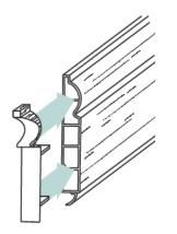
Measure from the flat face of skirting board 1 to the external corner of the wall. Cut the skirting board using square cuts. Fit a scribed internal corner moulding to the left hand end and check for fit. If satisfied fix in position with adhesive.
