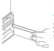
Measure length 2 from the flat face of the skirting board to the inside corner of the room. Cut to length using square cuts.
