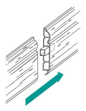
Push fit the in-line joint moulding so that half the moulding is inside the skirting and half protrudes.
