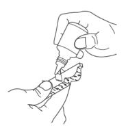
Apply adhesive to the external corner mouldings and push fit onto each end of length 3. Apply adhesive to the back face of the skirting board and the remaining tabs of the corner mouldings and fix into position making sure that the tabs locate into their correct position within the previously fitted lengths 2 & 4. Wipe off any surplus adhesive.
