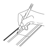
Measure length 1 from the external edge of the architrave to the inside corner of the room. Transfer this measurement onto a length of skirting board and mark accurately with a pencil. Cut the skirting board to length using square cuts with the aid of a fine toothed saw and saw block. Position the skirting board to check length.
