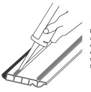
Lay the skirting board on its face and apply a bead of gap filling adhesive or another contact building adhesive down each adhesive channel. Place the skirting board in position pushing firmly back to the wall.
